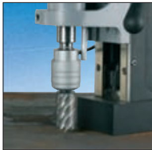
Drilling with core drills
