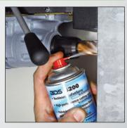
Step 2: During drilling, spray the high-performance lubrication spray onto the tip of the drill and into the borehole.
