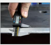
Chamfer width 30 mm max.
