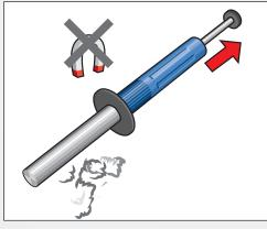
The chips can then be disposed of in a contact-less manner by demagnetisation.
