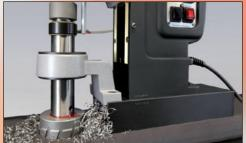
Magnetic core drilling with large calibres.
