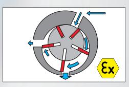
AirMAB 5000 – magnetic core drilling with pneumatic drive. The high performance vane motor performs at 830 Watt and is approved according to Ex class - Ex II 2G T4 IIC D110° C. See page 37.
