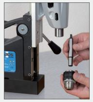
1. Connect taper drift to drill chuck.
