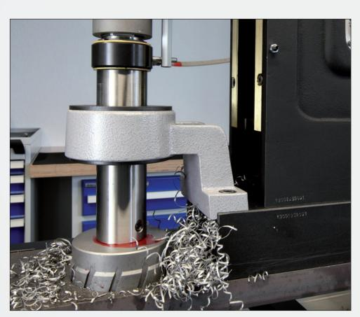
The MAB 1300 in its element: drilling, countersinking, reaming, thread cutting.
