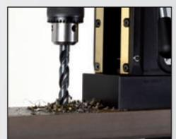
Twist drilling up to  $\varnothing$  31.75 mm
