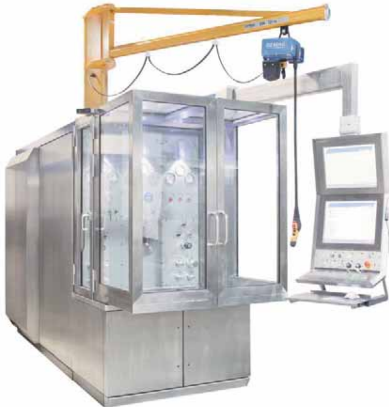
The figure shows a telescopic swivel arm, an operating unit with a second monitor, an integrated printer and pressure gauges
