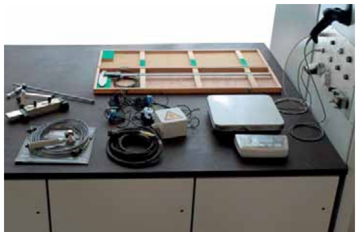
Additional Measuring Instruments (Scale, Sliding Caliper, Inclination Sensors, Bar Code Sensor)
