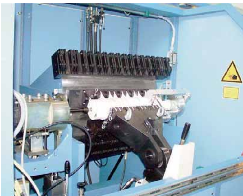
The picture shows the transmission unit with LEADING EDGE FLAP RH (P/N 2022636-4-4) F/A-18 mounted on it.
