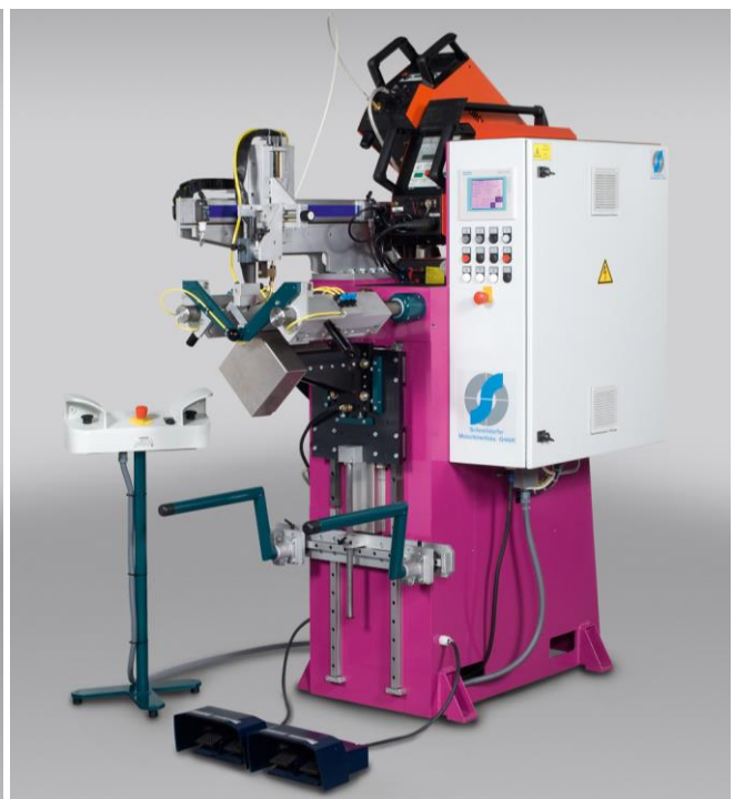
Figure 6: Mandrel lift up with clamped part
