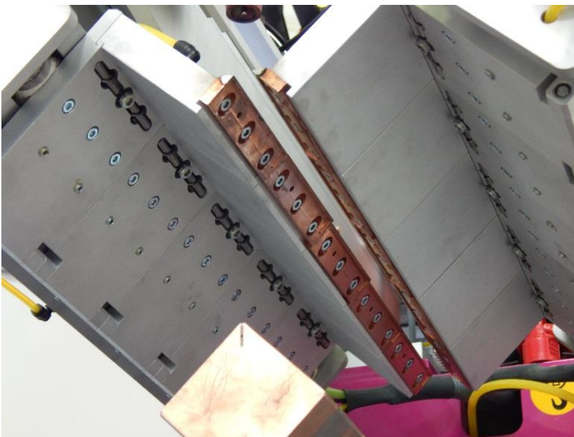
Figure 3: Flexible outside clamping system for outward bends up to 80 mm
