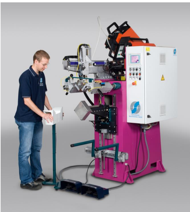
Figure 5: Mandrel lift down, Two-Hand-Control
