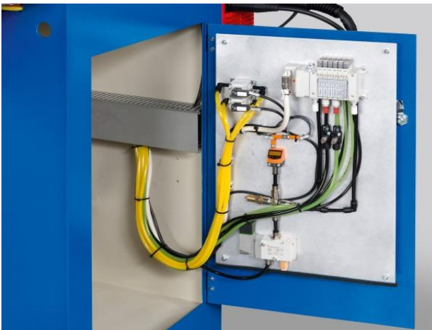
Figure 4: Pneumatics easily accessible from front of machine
