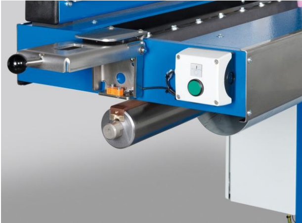
Figure 2: Manual latch open (position controlled, easy to operate)
