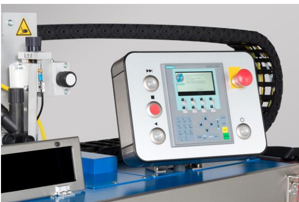
Figure 6: ELENA one control panel
